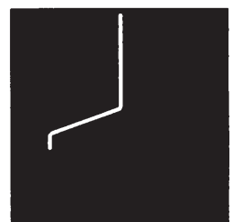
B-E paralleled by 680 \Omega
